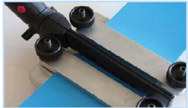
Welding narrow flat belts with Pliers P-200
