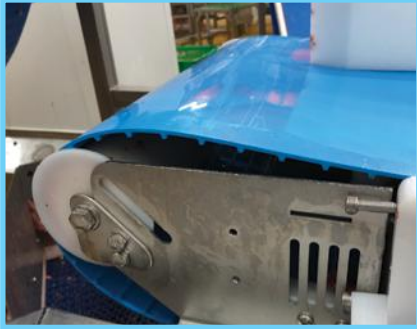
UHMW roundel mounted on pulley
