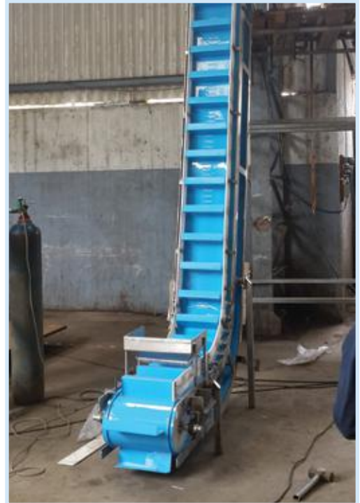
Fixed conveyor side wall
