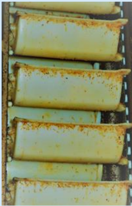
Open chain contaminated by food soil
