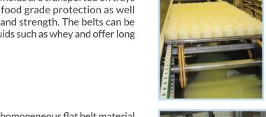
Hard Cheese: Volta's homogeneous flat belt material will not absorb water and oils and has no ply. Ply is prone to soak up liquids thereby developing high concentrations of bacteria and causing cracks to form in the laminated surface. Volta smooth surface belts can be scraped with no resulting damage to welded joints and no danger of grooving. Further fabrications such as flights and side walls for containment make this system adaptable to elevators and even swan-neck conveyors.
