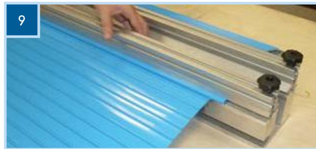
Position and tighten the FBW Crossbars. Weld the belt according to the FBW User Manual Instructions.
