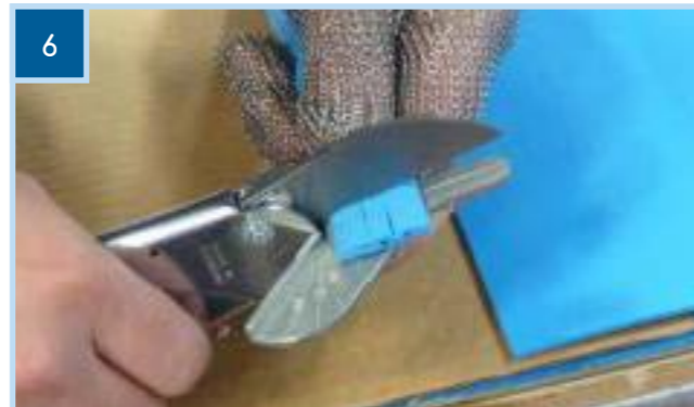
6 Cut the lace to the exact required width and use the markings previously made on the belt to aid this.
