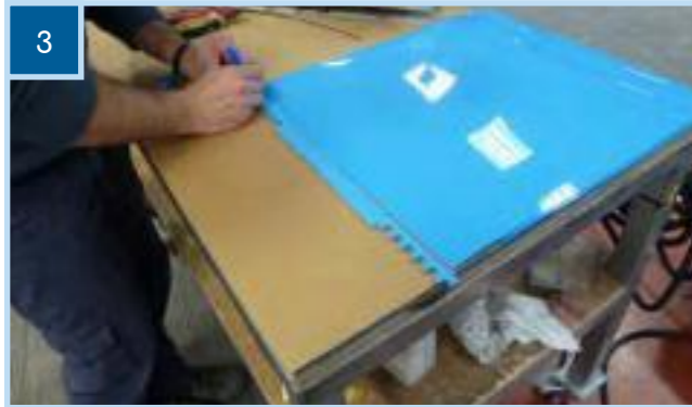
3 Mark the desired lace position (both ends) on the belt and take into account the indent described above.
