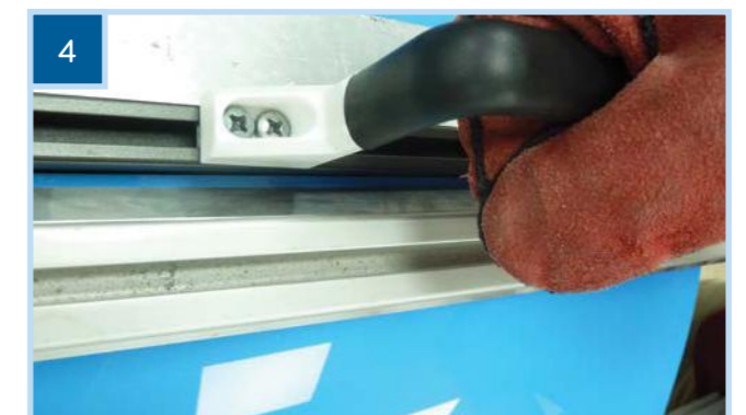
4 Weld the belt to the lace according to the welding instructions for FBW. The thicker the belt, the longer the melt should be to match the thickness of your belt.
