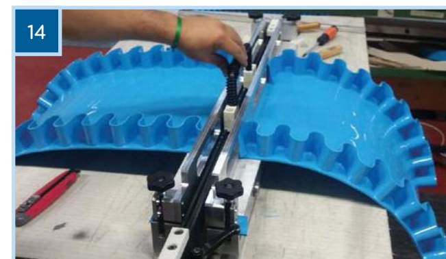
Welding the belt Weld the belt using a welder with the SW welder handle (Figure 14). For DD belts use the stoppers to keep the correct pitch.
