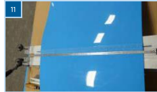
11 Position the second belt edge. Note that the first edge and lace are in position.
