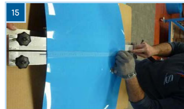
15 Mesh the pin and bend the edges over. The finished lace should look like this.
