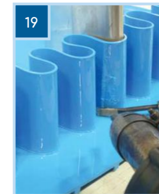
Re-Welding the Sidewalls Re-Weld the Sidewall to the belt using a hot air gun (Figure 19 & 20).
