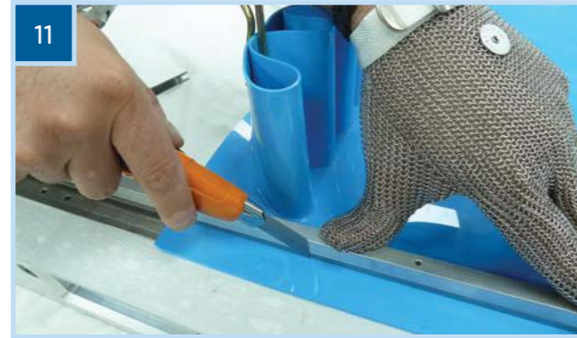
Cutting the belt Cut the belt along the Cutting Bar using a sharp utility knife (Figure 11). Repeat the procedure to cut the second side of the belt.
