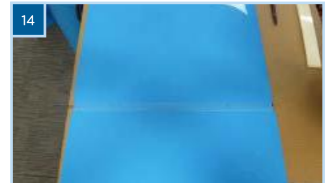
14 Now cut the belt edges to form the indent mentioned at the beginning of the lace instructions.
