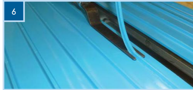
Rub a small amount of soap on the MiniCleave and on the blade of the straight trim knife (see figure 11). Close the FBW sides to use the second adapter as an anvil while carefully cutting the MiniCleave away from the belt.
