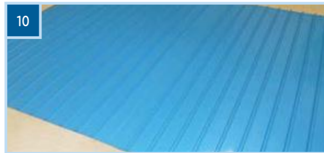
Trim and check the weld. A good weld will be free of cracks and defect. Pitch tolerance should be +0.0 mm, -1.0 mm.
