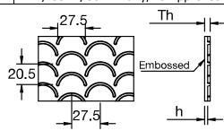
Coefficient of friction (Dry): Belt Embossed Bottom -Steel: 0.25
