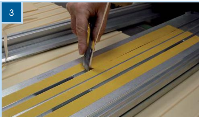
3 Apply Double-side Tape on the Adaptor surface and trim the unnecessary tape from the grooves. At this stage do not remove the protective paper.
