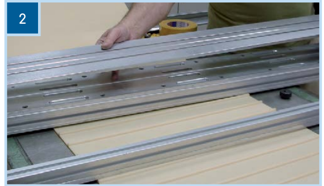
2 Select the appropriate adaptor for the belt type to be welded. Position the Adaptor onto the pliers when the groove of the electrode is facing up.
