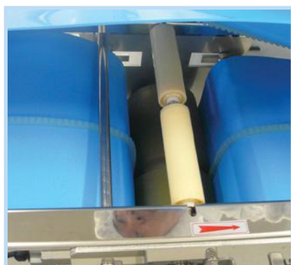
1. A single center guide on the underside of the belt used to prevent off-tracking.
