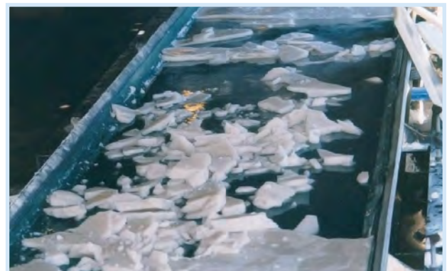
FZ-5: CONVEYING CAUSTIC SODA
