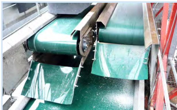
FRPZ-6 with Hammocks : PLASTIC PARTS CONVEYING
