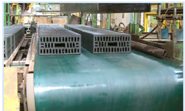
FRZ-4: HEAVY BRICK CONVEYING
