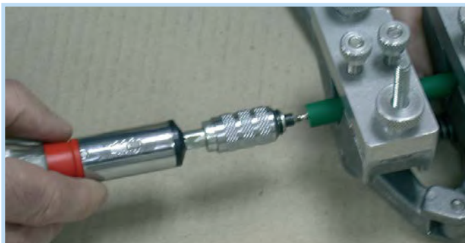
3a. When welding reinforced V and Round profiles, place one end of the belt in the Pliers (as shown above) so that it protrudes 5-10 mm from the Pliers. Using the D-11 Driller and correct diameter bit, drill out the reinforcement cord until it is at full depth. Repeat for opposite end of belt.
