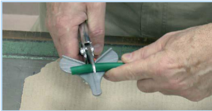
1. Using the Lowe Belt Snipper, cut the belt to the desired length. Both ends should be cut straight.
