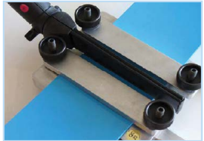
Welding narrow flat belts with Pliers P-200
